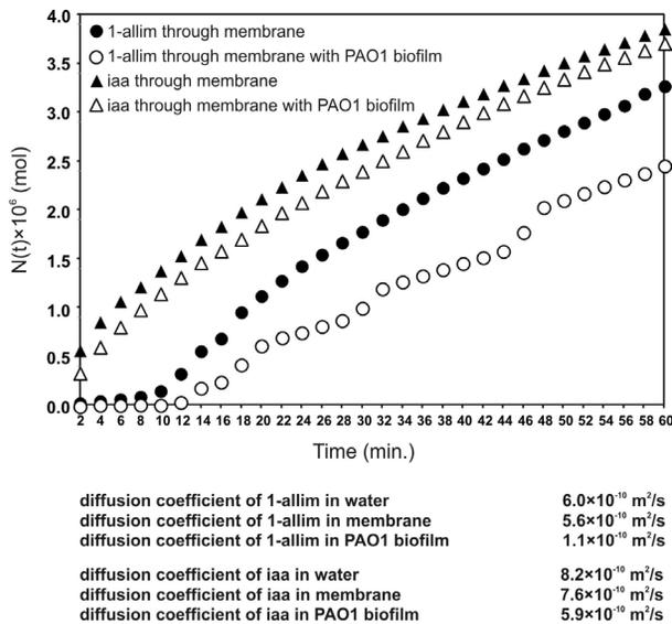
Figure 2. The laser interferometry analysis of 1-allylimidazole or imidazole-4-acetate anion diffusion through PAO1 biofilm formed on Nephropane membrane for 72 h, at 37°C, 5% CO<sub>2</sub>, as well as the native membrane.
