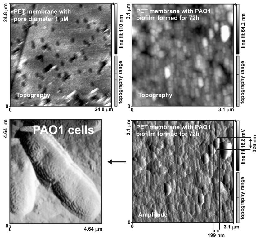
Figure 4. Topography and amplitude of PET membrane alone and with PAO1 biofilm formed for 72 h, at 37°C, 5% CO<sub>2</sub>, measured by AFM microscopy.
