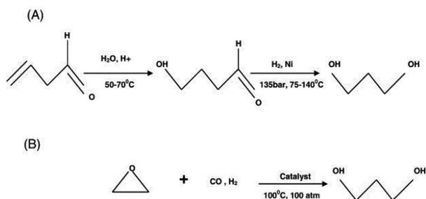
**Figure 3.** Chemical synthesis of 1,3-PDO : A) from acrolein, B) from ethylene oxide (Lawrence & Sullivan, 1972; Chuah *et al.*, 1995).
