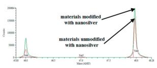
Figure 6. Mass spectrum showing the comparison of the intensity of Ti (<sup>46</sup>Ti, <sup>47</sup>Ti, <sup>48</sup>Ti) ions released from X Flow Demi composite unmodified and modified with nanosilver stored at 37°C after three months of incubation.
