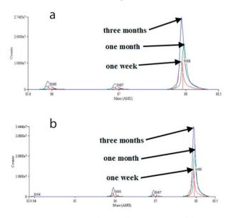
Figure 5. Mass spectrum showing the comparison of the intensity of Sr (<sup>86</sup>Sr, <sup>87</sup>Sr, <sup>88</sup>Sr) ions released from Dyfract Fow Demi compomer modified with nanosilver stored at (a) room temperature and (b) 37°C after a week, a month and three months of incubation.
