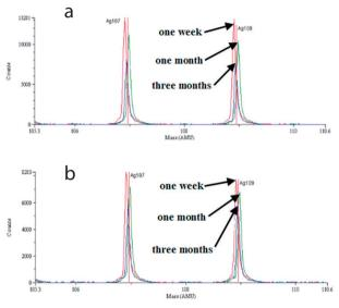
Figure 7. Mass spectrum showing the intensity Ag peaks for (a) X Flow Demi and (b) Dyfract Flow modified with nanosilver vs. incubation time at human body temperature.
