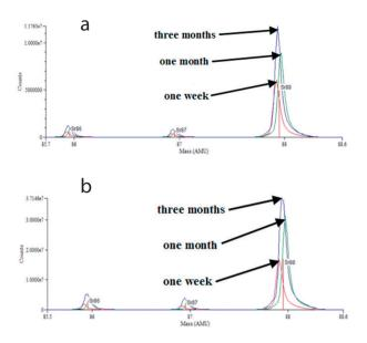
Figure 4. Mass spectrum showing the comparison of the intensity of Sr ( $^{\infty}$ Sr,  $^{\infty}$ Sr,  $^{\infty}$ Sr) ions released from X Flow Demi modified with nanosilver stored at (a) room temperature and (b) 37°C after a week, a month and three months of incubation.
