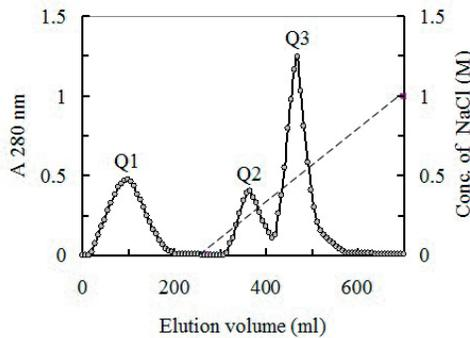
**Figure 1.** Ion exchange chromatography on Q-Sepharose.
