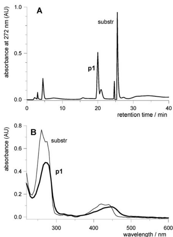
**Figure 6.** HPLC chromatogram (A) (reversed phase, methanol + water gradient system, 272 nm) taken after 16-h incubation of  $10^{-4}$  M 2-hydroxyacridinone with  $0.0005 \mu\text{g/ml}$  HRP and  $10^{-4}$  M  $\text{H}_2\text{O}_2$ ; and UV-VIS spectra (B) collected for HPLC peaks of substrate and p1.
