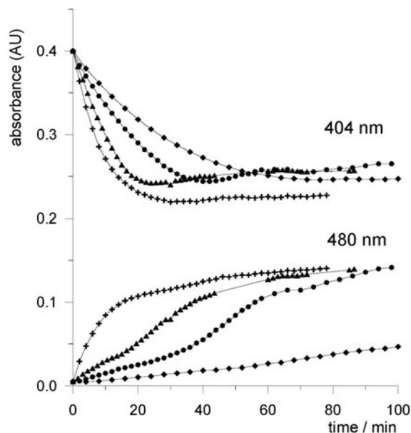
**Figure 5.** Time dependence of the absorbance at 404 and 480 nm during the incubation of  $10^{-4}$  M 2-hydroxyacridinone with  $0.005 \mu\text{g/ml}$  HRP and with compound : H<sub>2</sub>O<sub>2</sub> ratios:  $\square$  1 : 5;  $\blacktriangle$  1 : 2;  $\bullet$  1 : 1 and  $\blacklozenge$  1 : 0.5.
