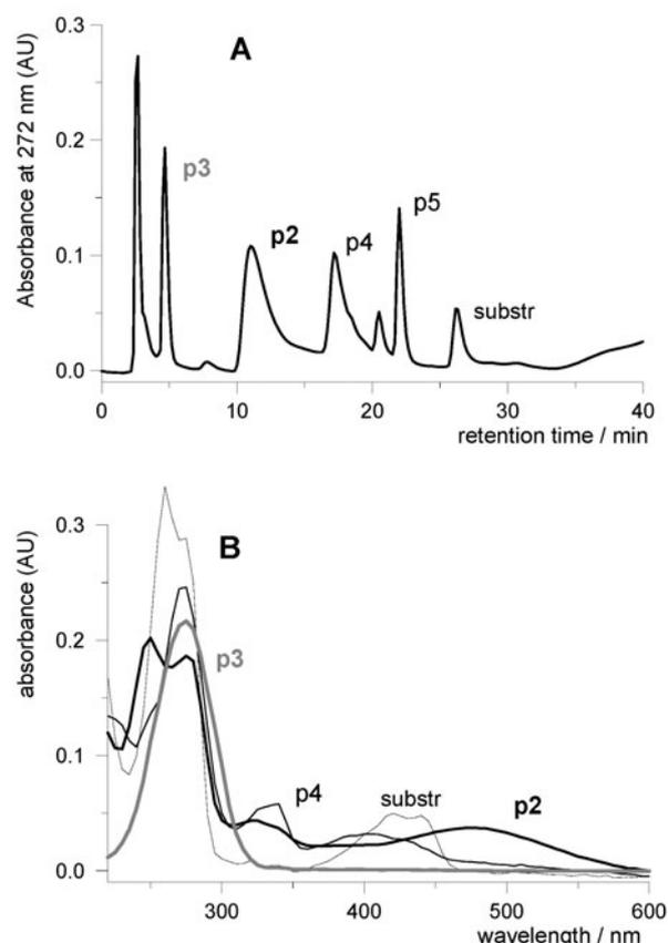
**Figure 7.** HPLC chromatogram (A) (reversed phase, methanol + water gradient system, 272 nm) taken after 16-h incubation of  $10^{-4}$  M 2-hydroxyacridinone with  $0.005 \mu\text{g/ml}$  HRP and  $10^{-4}$  M  $\text{H}_2\text{O}_2$ ; and UV-VIS spectra (B) collected for HPLC peaks of substrate and products p2, p3 and p4.
