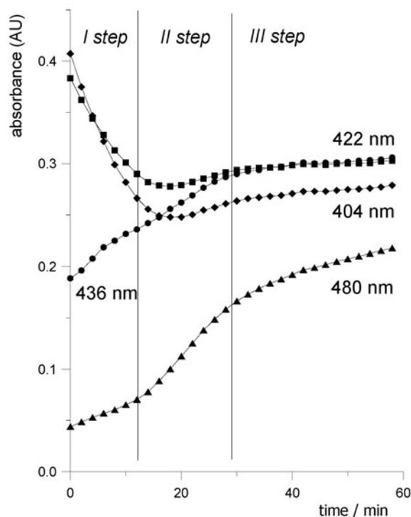
Figure 3. Time dependence of the absorbance at 404, 422, 436 and 480 nm during the incubation of  $10^{-4}$  M 2-hydroxyacridinone with equimolar amount of  $\text{H}_2\text{O}_2$  and 0.01  $\mu\text{g/ml}$  of HRP.
