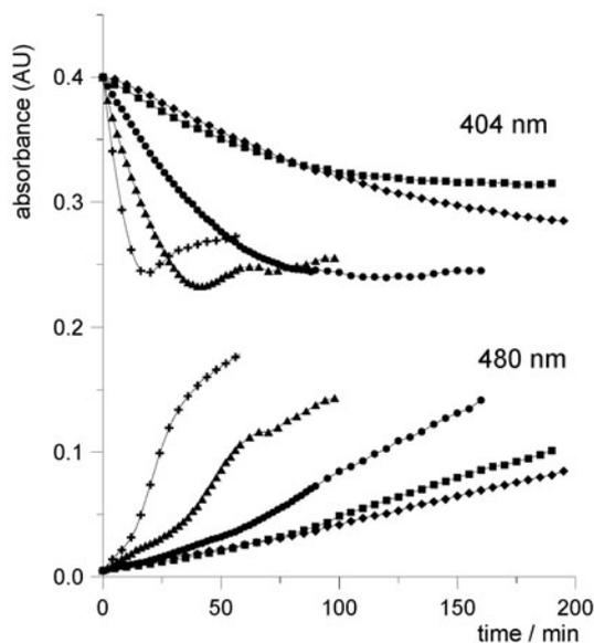
Figure 2. Time dependence of the absorbance at 404 and 480 nm during the incubation of  $10^{-4}$  M 2-hydroxyacridinone with equimolar amount of  $\text{H}_2\text{O}_2$  and various HRP concentrations: + 0.01  $\mu\text{g/ml}$ ;  $\blacktriangle$  0.005  $\mu\text{g/ml}$ ;  $\bullet$  0.002  $\mu\text{g/ml}$ ;  $\blacksquare$  0.001  $\mu\text{g/ml}$  and  $\blacklozenge$  0.0005  $\mu\text{g/ml}$ .
