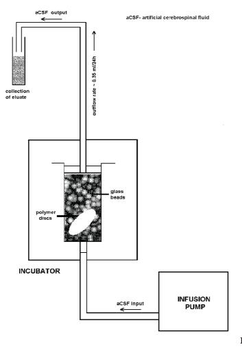
Figure 1. Schematic diagram of the experimental system.
